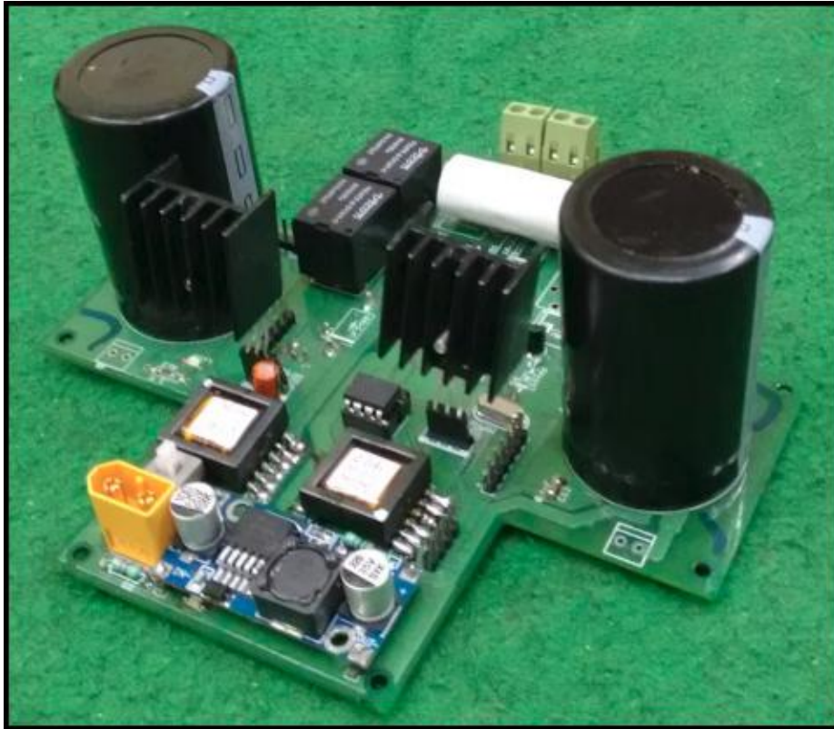
Fig. 5. Final fabricated Kicker circuit
